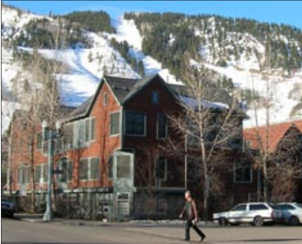
Subdivide the mass of a building into smaller “modules” that convey a human scale.
