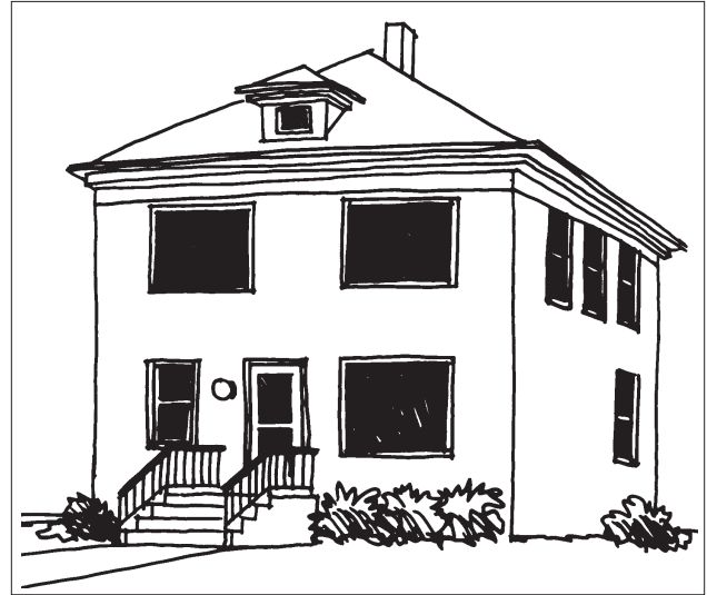
This is an inappropriate remodel. The porch on this house has been removed and the original windows have been replaced with new windows that are out of scale.
