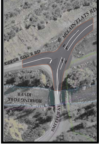
Aerial View of Modified “T” Intersection
